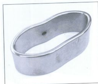
Figure 4. Steel test ring with a 50 microns Hardide coating crushed to test coating adhesion and toughness – no flaking or coating separation from the substrate.
