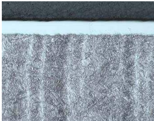
Fig. 6. Pore-free Hardide™ coating protects the substrate against aggressive media attacks; a micro-graph of a Hardide-coated sample of 17-4 stainless steel after 30 days in solution of NaCl, Acetic Acid and H 2 S (micro-photograph from Bodycote report [9]).
