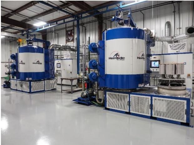
**Hardide developed and commercialised a patented CVD tungsten carbide nano-structured coating with a unique combination of properties**
